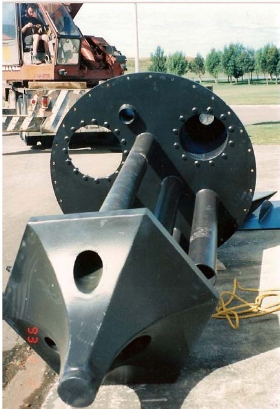
Figure 3: Central eductor tube and deflector cone in the current digester mixing system used to mix the digester and to splash/spread mixed liquor onto top of scum layer to reduce scum formation.
